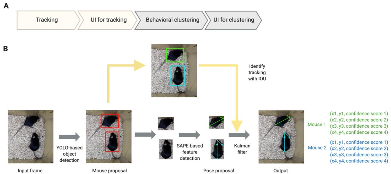
**Figure 1: AlphaTracker architecture and pipeline** **A.** Overview of the AlphaTracker pipeline. **B.** architecture of AlphaTracker which combines object detection using You Only Look Once (YOLO) neural network, pose estimation using Single Animal Pose Estimation (SAPE), and identity tracking based on intersection over union (IOU) for subsequent frames with an additional Kalman filter to correct tracking errors.
